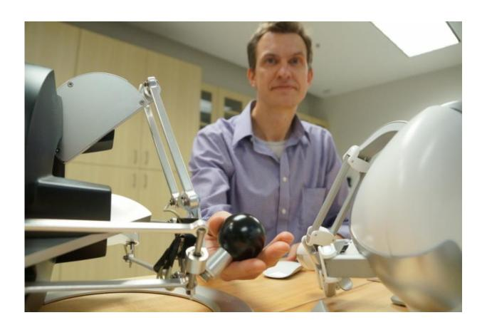
UCSB researcher Yon Visell and a device of the type used to simulate the forces felt by the hand when touching an object. Credit: Sonia Fernandez
