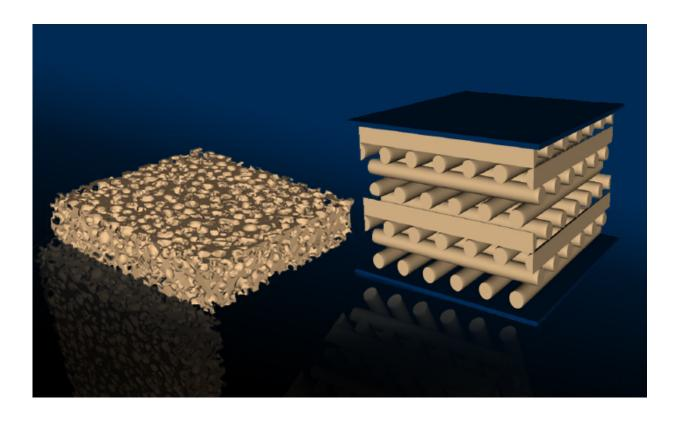
Microstructures of two different foam materials. At left, a traditional open-cell stochastic foam, and a right, a 3D printed foam with the face-centered tetragonal lattice structure.
