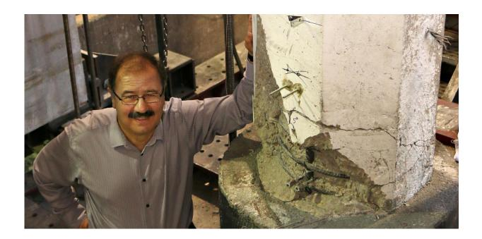
University of Utah civil and environmental professor Chris Pantelides stands next to a donut-sized "repair" he and a team of researchers designed that can fix a damaged column on a bridge. The repair -- a black concrete donut surrounding the ends of the column and wrapped with a composite fiber material -- can be deployed on bridges damaged in an earthquake much more quickly than through the standard procedure. Credit: University of Utah College of Engineering
