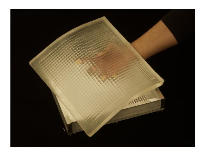
Columbia Engineering researchers have developed a novel sheet camera that can be wrapped around everyday objects to capture images that cannot be taken with one or more conventional cameras. They designed and fabricated a flexible lens array that adapts its optical properties when the sheet camera is bent. This optical adaptation enables the sheet camera to produce high quality images over a wide range of sheet deformations. Credit: Columbia Computer Vision Laboratory,
