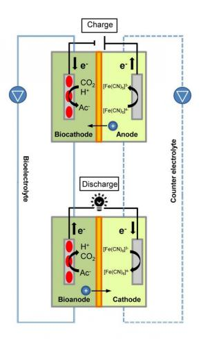
The microbial rechargeable battery consists of a charging cell (performing microbial electrosynthesis) and discharging cell (the microbial fuel cell). Credit: Molenaar, et al. ©2016 American Chemical Society
