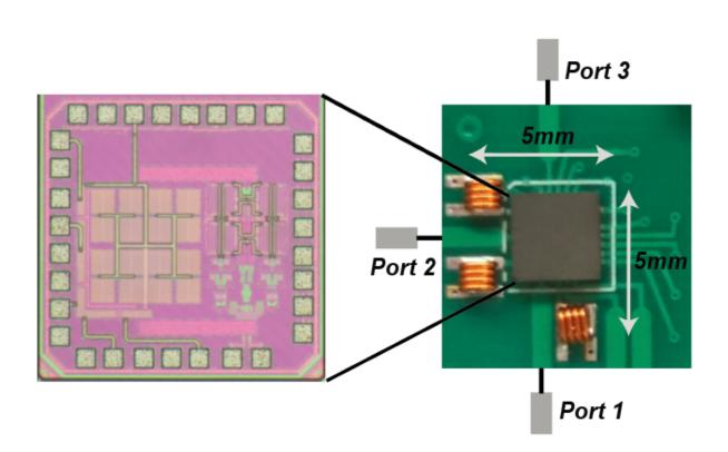
The microphotograph of the CMOS circulator IC along with a close-up photograph of the packaged IC on a printed circuit board. Credit: Negar Reiskarimian, Columbia Engineering
