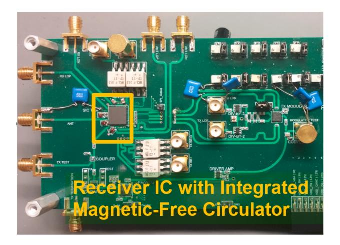
The first CMOS full duplex receiver IC with integrated magnetic-free circulator. Credit: Negar Reiskarimian, Columbia Engineering
