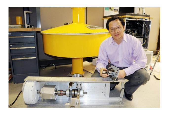
Lei Zuo holds the first version of the wave energy harvester, while a larger version of the device sits at his feet. When in use, the harvester will be encased in a yellow buoy like the one behind him. Credit: Virginia Tech
