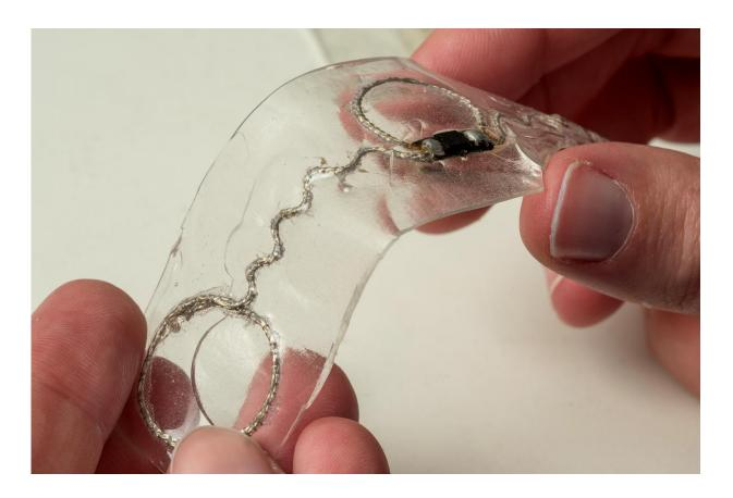
Researchers at The Ohio State University are developing embroidered antennas and circuits with 0.1 mm precision -- the perfect size to integrate electronic components such as sensors and computer memory devices into clothing. They are also exploring other uses for the technology, including this flexible circuit that contains an RFID chip. Credit: Jo McCulty, courtesy of The Ohio State University
