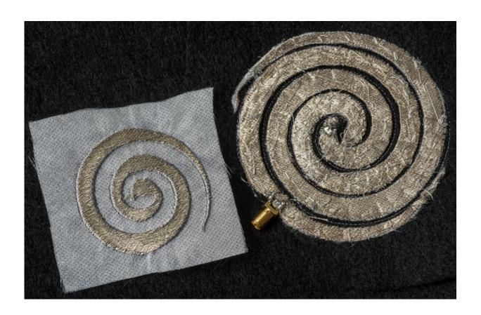
Researchers at The Ohio State University are developing embroidered antennas and circuits with 0.1 mm precision—the perfect size to integrate electronic components such as sensors and computer memory devices into clothing. Credit: Jo McCulty, courtesy of The Ohio State University.
