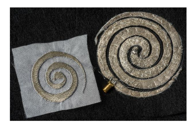
Researchers at The Ohio State University are developing embroidered antennas and circuits with 0.1 mm precision—the perfect size to integrate electronic components such as sensors and computer memory devices into clothing. Credit: Jo McCulty, courtesy of The Ohio State University.
