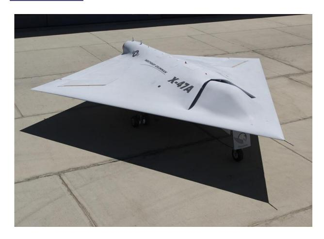
The Northrop Grumman X-47A Pegasus drone is being trialed by the US Navy. Credit: DARPA
