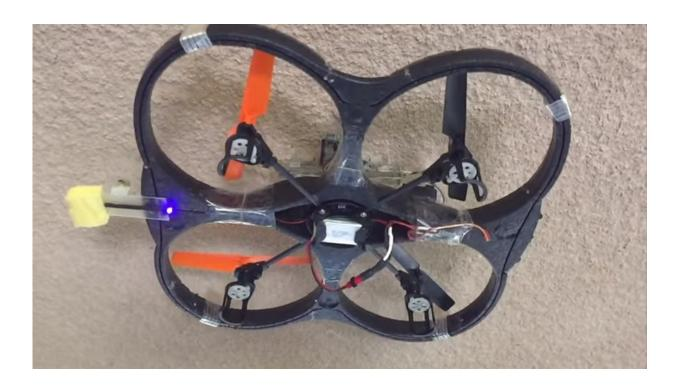
Researchers at Stanford's Biomimetics and Dexterous Manipulation Lab investigate robots at the boundary of airborn and surface locomotion. They have made a drone that, like insects, can land on vertical walls and even ceilings. This addresses a problem with hovering drones—namely, endurance.
