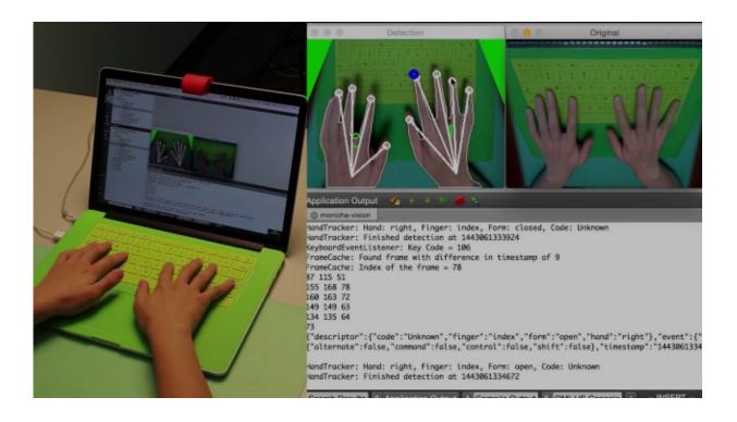
Researchers evaluate and demonstrate finger, hand, and posture identification as keyboard shortcuts. By detecting the hand and finger used to press a key, and open or closed hand postures, a key press can have multiple command mappings.
