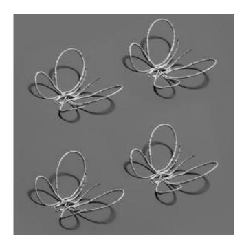
Laser-assisted direct ink writing allowed this delicate 3D butterfly to be printed without any auxiliary support structure. Credit: Lewis Lab/Harvard University
