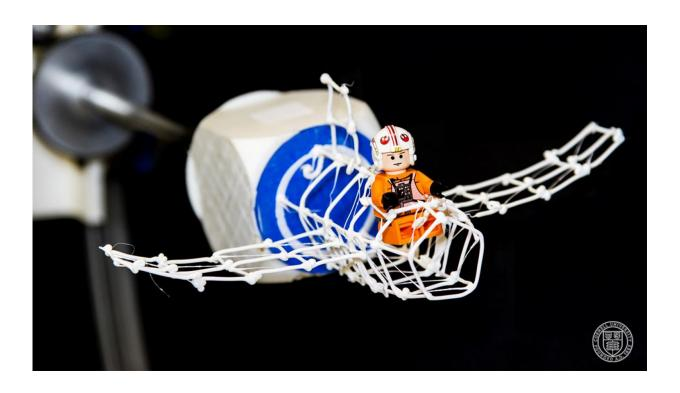
This wire frame prototype of a toy aircraft was printed in just 10 minutes, including testing for correct fit, and modified during printing to create the cockpit. The file was updated in the process, and could be used to print a finished model. Credit: Cornell University
