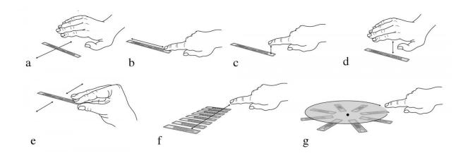
Types of interaction with RFID tags include: (a) wave; (b) swipe; (c) finger touch; (d) cover touch; (e) free air tag motion; (f) slider; (g) knob. Credit: Eric Brockmeyer/Disney Research
