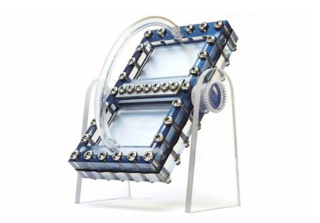
A new concept for a flow battery functions like an old hourglass or egg timer, with particles (in this case carried as a slurry) flowing through a narrow opening from one tank to another. The flow can then be reversed by turning the device over.
