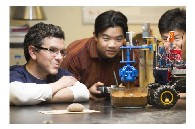
The device was attached to a remote-controlled small rover. The researchers first tested the claw on beach sand, where it performed well. They then used the claw on sand that simulates Martian soil in density and humidity (or lack thereof). The device was able to scoop up sand efficiently. Credit: Jacobs School of Engineering/UC San Diego
