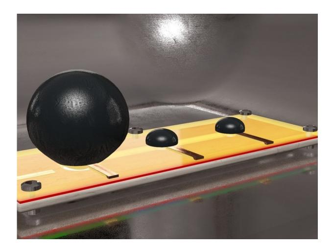
Elastic machines: Membranes surrounding sealed, air-filled chambers can be used as actuators, facilitating risk-free contact between humans and robots. Compliant electrodes are attached to each side of the membrane and cause it to stretch when voltage is applied. The membranes are bistable, meaning that they
