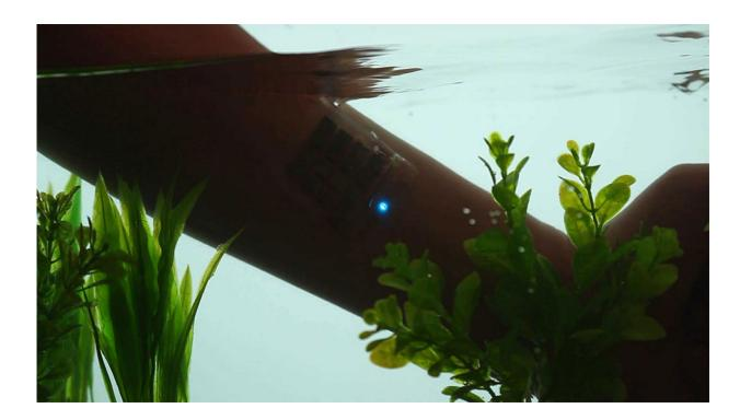
Soft, stretchable power storage device connected to an LED, laminated onto the forearm and submerged in water. Credit: J. Rogers, University of Illinois.
