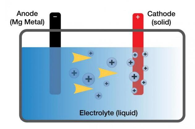
Batteries are made up of three main components: a ANODE (-), a CATHODE (+) and between them, a ELECTROLYTE. Electrons move between the anode and the cathode through the external circuit, while ions are transported through the electrolyte to balance the charge. Different metal combinations require different electrolytes that must efficiently allow the movement of ions while not corroding the anode and cathode.
