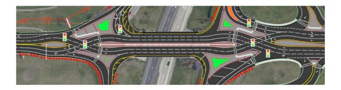
Overview of Diverging Diamond Interchanges, or DDIs, that divert drivers to the left side of the road prior to merging onto an interstate, freeway or highway. Credit: Carlos Sun
