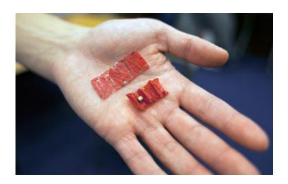
The new robot consists of two layers of structural material sandwiching a material that shrinks when heated. A pattern of slits in the outer layers determines how the robot will fold when the middle layer contracts. Credit: Melanie Gonick/MIT
