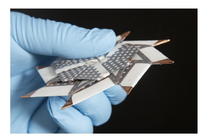
This new disposable battery, developed at Binghamton University, folds like an origami ninja star and could power biosensors and other small devices for use in challenging field conditions. Credit: Jonathan Cohen/Binghamton University
