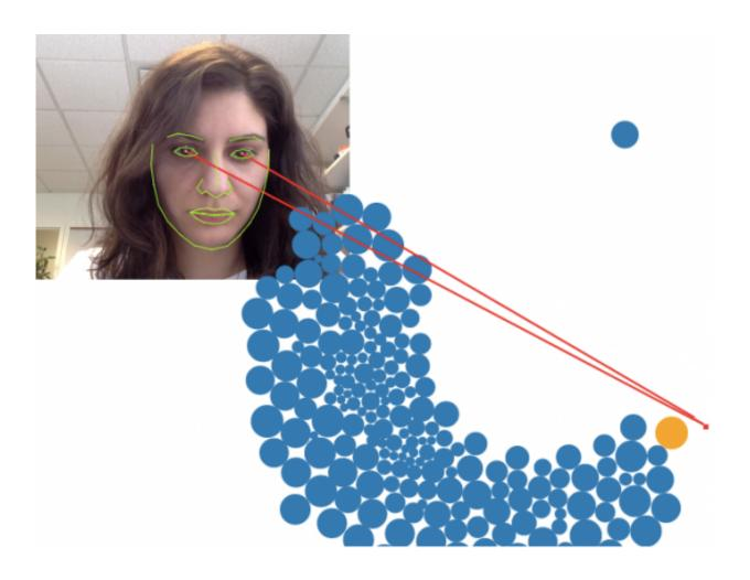
Eye-tracking helps web developers make better websites, but it's expensive to do. New software, which can be embedded in any website, turns webcams into eye trackers. Credit: Huang Lab / Brown University
