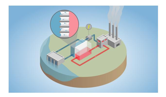
The temperature difference between a waste heat source and the environment drives water across the nanobubble membrane (enlarged) and through a turbine to generate electricity. Credit: Yale University
