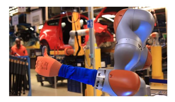
New collaborative robots, also known as co-bots, are first being used to help workers fit shock absorbers to Fiesta cars, a task that requires pinpoint accuracy, strength, and a high level of dexterity. Employees work hand-in-hand with the robots to ensure a perfect fit every time. Credit: Ford Motor Company
