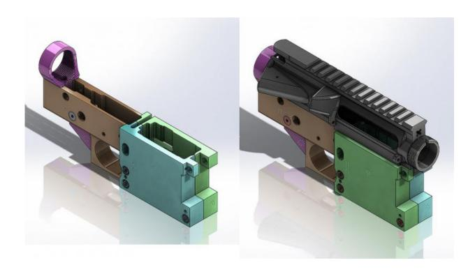
A computer design for home manufacturing of a receiver, the trigger and firing part, of a semi-automatic rifle. Credit: simonov/flickr, CC BY-SA
