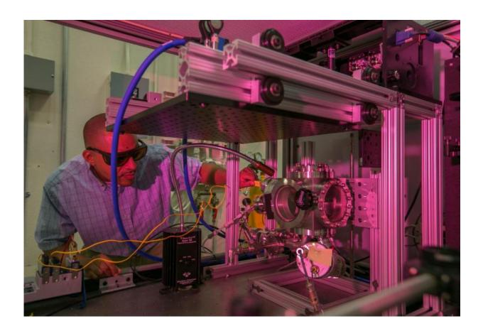
Ibo Matthews inspects an in situ diagnostics test bench his team developed for studying laser-driven powder bed fusion additive manufacturing. High-speed thermal and optical mapping of the laser-powder interaction has enabled the team to reveal new physics associated with the process and helped guide highperformance computing simulations. Credit: Julie Russell
