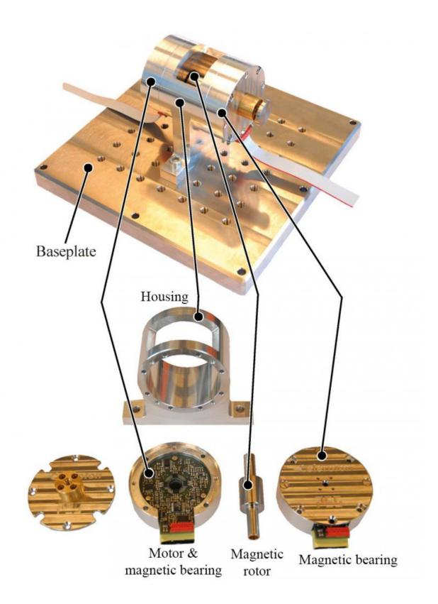
Components of the reaction wheel motor and their assemblage. Credit: Zwyssig
