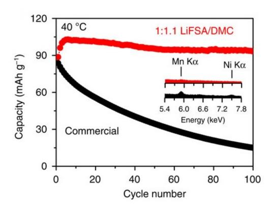
A battery with the new superconcentrated electrolyte (red line) has a capacity retention of more than 90% over 100 cycles, whereas a battery with a common commercial electrolyte (black line) has a capacity retention of less than 30% over 100 cycles. Credit: Wang et al. Nature Communications
