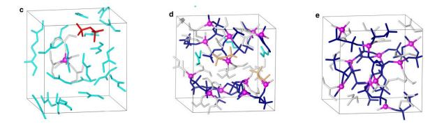
Chemical structures and equilibrium trajectories of electrolyte solutions that are (left) dilute, (center) moderately concentrated, and (right) superconcentrated. The superconcentrated solution has a reinforced 3D network structure that prevents negatively charged ions from bonding with and dissolving the positively charged aluminum ions in the current collector. Credit: Wang et al. Nature Communications
