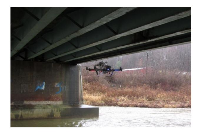
Northeastern's Jerome Hajjar and colleagues are developing a sophisticated system that uses autonomous small flying robots coupled with 3-D imaging and state-of-the art planning, modeling, and analysis to inspect structures from bridges to buildings and automatically identify problems, track their progress, and assess the need for follow-up. Credit: Varun Kasireddy/Carnegie Mellon University
