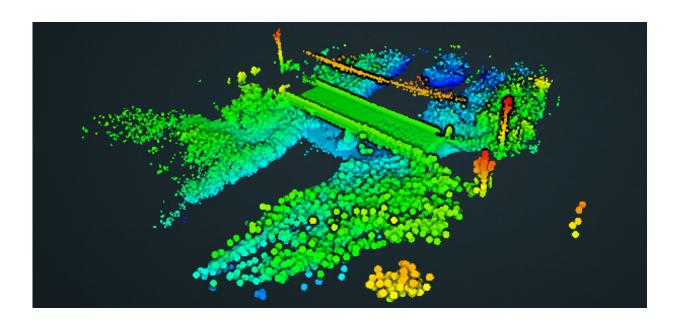
An overview of a 3-D model of a bridge created by the autonomous ARIA robot using its unique sensors. Credit: Varun Kasireddy, Carnegie Mellon University
