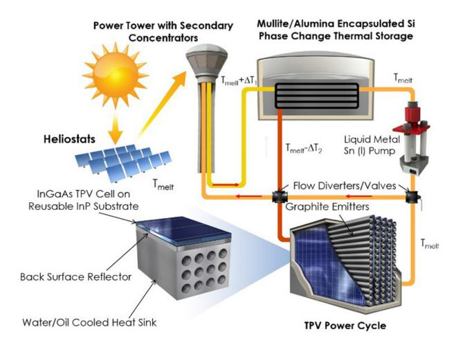
This schematic shows a thermophotovoltaic system that would be used to convert high-temperature heat from concentrated solar thermal to utility-scale electricity. Credit: Hamid Reza Seyf
