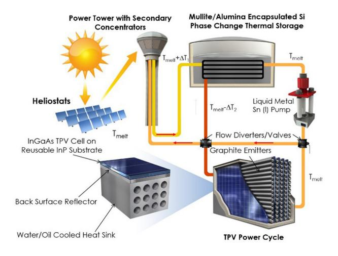
This schematic shows a thermophotovoltaic system that would be used to convert high-temperature heat from concentrated solar thermal to utility-scale electricity. Credit: Hamid Reza Seyf
