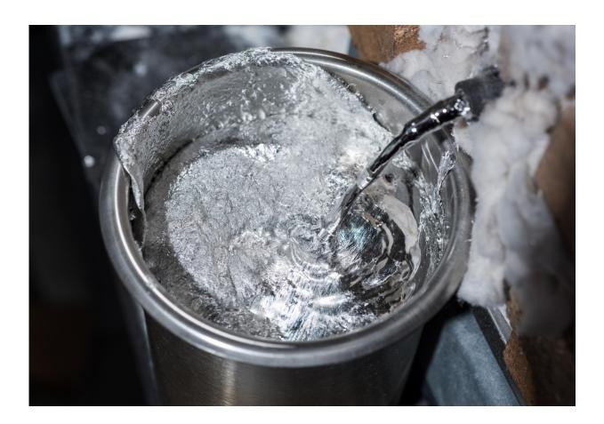
Researchers in the laboratory of Asegun Henry at Georgia Tech are developing a thermal storage system that uses liquid tin as a transport fluid. The storage medium itself would be metallurgical grade silicon or an aluminum silicon alloy, which is much more cost effective. The technology they have developed could help increase the efficiency of energy systems based on concentrated solar thermal energy. Credit: Rob Felt, Georgia Tech
