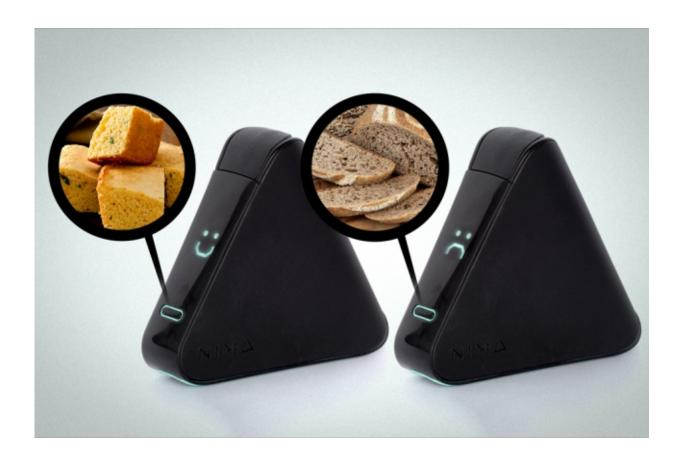
To use the Nima sensor, a new device that can detect gluten, diners put a peasized sample of food or liquid into a disposable capsule, and insert the capsule into the device, which mixes the food into a solution that detects gluten. In two to three minutes, a digital display appears on the sensor, indicating if the food sample does or doesn't contain gluten. Credit: MIT News
