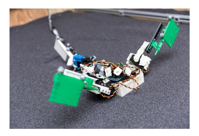
Image shows a robot that used the locomotion principles of the mudskipper to move through a trackway filled with granular materials. The robot has two limbs and a powerful tail, with motion provided by electric motors. Credit: Rob Felt, Georgia Tech
