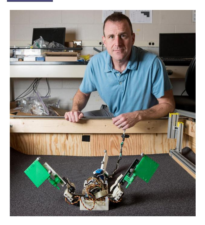
Dan Goldman, associate professor in the Georgia Tech School of Physics, is shown with the "MuddyBot" robot in a trackway used to study how the robot which was modeled on the mudskipper fish - moved across granular surfaces. Credit: Rob Felt, Georgia Tech
