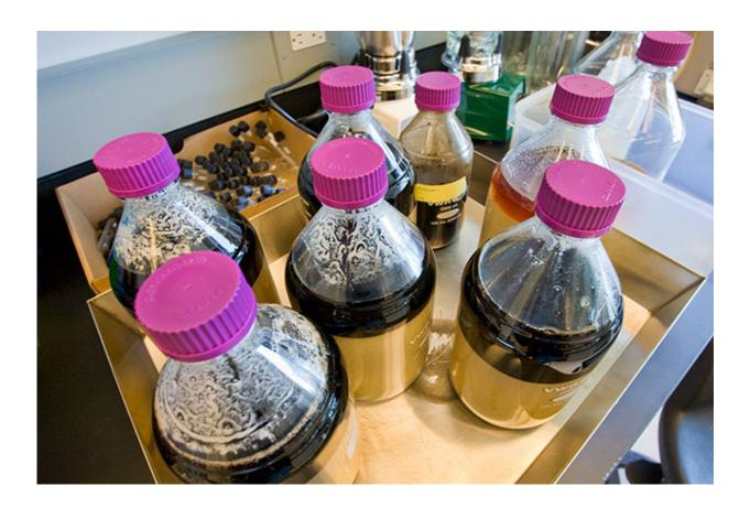
JBEI scientists have advanced the use of ionic liquids, shown here, to break down cellulosic biomass. The latest development involves the use of carbon dioxide to reversibly adjust the pH level of ionic liquids, greatly simplifying the biofuel production process and lowering cost. Credit: Roy Kaltschmidt/Berkeley Lab
