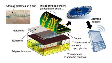
Threads penetrate multiple layers of tissue to sample interstitial fluid and direct it to sensing threads that collect data, such as pH and glucose levels. Conductive threads then deliver the data to a flexible wireless transmitter sitting on top of the skin. The inset figure, upper left, shows liquid flowing in threads sutured into
