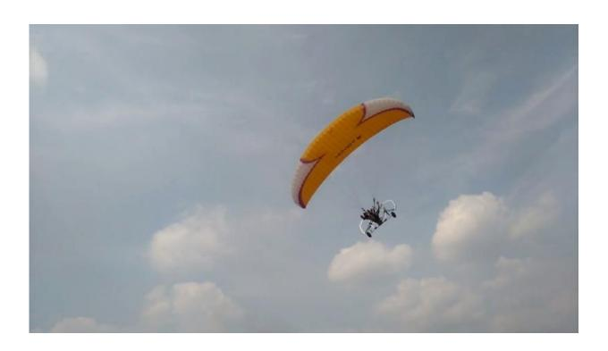
The Delta weighs just 49 kilogrammes, can fly up to a speed of 36 kilometres per hour under normal wind conditions, and for a typical flight time of 10 minutes on fully-charged batteries. Credit: National University of Singapore
