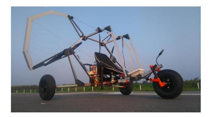
The Delta's form is simple, minimalistic, yet sturdy – it has a chassis with wheels and steering, a seat for the driver, two electric motors, two propellers, and it incorporates an off-the-shelf paraglider. Credit: National University of Singapore
