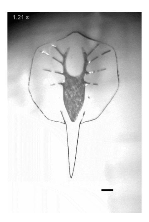
Upon optical stimulation, the tissue-engineered ray propelled by producing forward thrust via the undulatory motion of its fins. Credit: Sung-Jin Park
