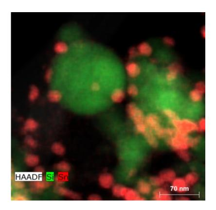
The silicon-tin nanocomposite developed at UCR viewed by high angle angular dark field imaging. The larger green particles are silicon and the smaller red particles are tin. Credit: UC Riverside
