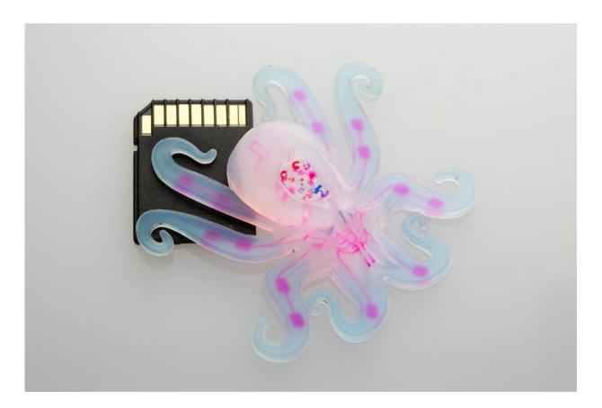
The octobot is powered by a chemical reaction and controlled with a soft logic board. A reaction inside the bot transforms a small amount of liquid fuel (hydrogen peroxide) into a large amount of gas, which flows into the octobot's arms and inflates them like a balloon. The team used a microfluidic logic circuit, a soft analog of a simple electronic oscillator, to control when hydrogen peroxide decomposes to gas in the octobot. Credit: Lori Sanders
