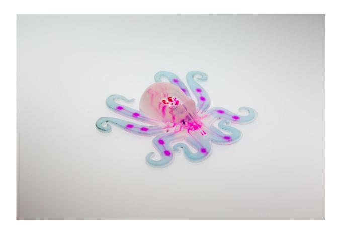
The octobot is powered by a chemical reaction and controlled with a soft logic board. A reaction inside the bot transforms a small amount of liquid fuel (hydrogen peroxide) into a large amount of gas, which flows into the octobot's arms and inflates them like a balloon. A microfluidic logic circuit, a soft analog of a simple electronic oscillator, controls when hydrogen peroxide decomposes to gas in the octobot. Credit: Lori Sanders
