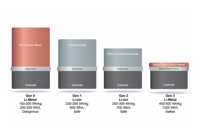
SolidEnergy Systems' battery (far right) is twice as energy-dense, yet just as safe and long-lasting as the lithium ion batteries used in consumer electronics. The battery uses a lithium metal foil for an anode, which can hold more ions and is several times thinner and lighter than traditional lithium metal, graphite, carbon, or silicon anodes. A novel electrolyte also keeps the battery from heating up and catching fire. Credit: SolidEnergy Systems
