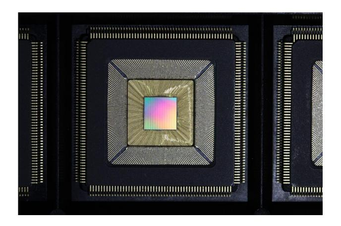
Unlidded Princeton Piton Processor. Multicolored die is wirebonded inside chip package. Credit: Princeton University
