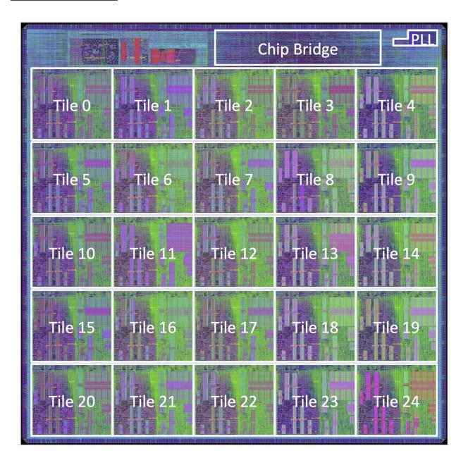
An annotated CAD tool layout of the Princeton Piton Processor showing 25 cores. Credit: Princeton University
