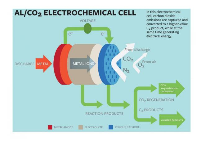
This graphic explains novel method for capturing the greenhouse gas and converting it to a useful product -- while producing electrical energy. Credit: Cornell University
