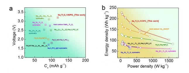
The sodium-ion full cell reported here is one of the top-performing sodium-ion full batteries in terms of several factors, including voltage, capacity, energy density, and power density. Credit: Hongsen Li et al. ©2016 The Royal Society of Chemistry
