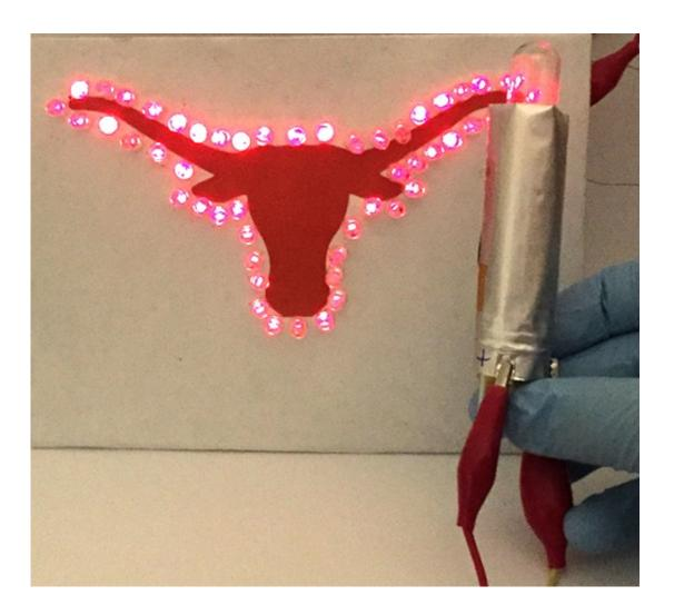
The rolled sodium-ion full-cell battery is shown powering an array of red LEDs in the outline of a longhorn, the logo of the University of Texas at Austin. Credit: Hongsen Li et al. ©2016 The Royal Society of Chemistry
