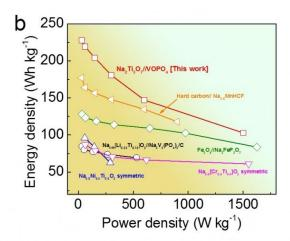
The sodium-ion full cell reported here is one of the top-performing sodium-ion full batteries in terms of several factors, including voltage, capacity, energy density, and power density. Credit: Hongsen Li et al. ©2016 The Royal Society of Chemistry
