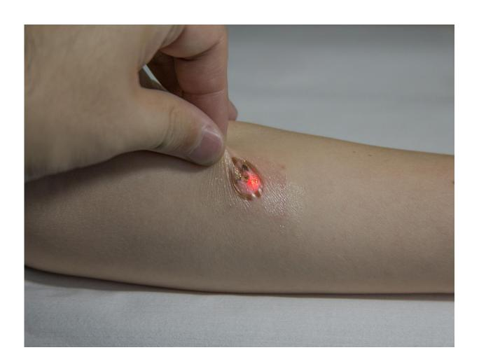
An image of the lighting red LED of the pulse rate monitoring device mounted on skin. Credit: Kim et al.
