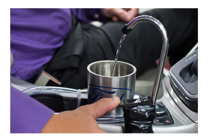
Ford's prototype On-the-Go H2O system collects, filters and pumps water directly to a faucet hanging over the cupholders.
