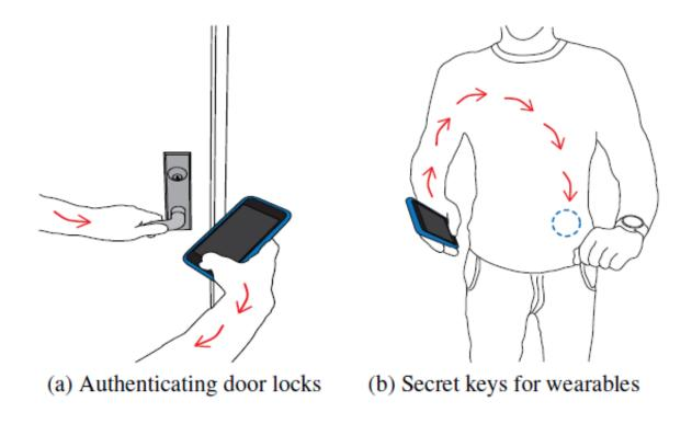
Potential applications for on-body transmissions include securely sending information to door locks, glucose sensors or other wearable medical devices. Credit: Vikram Iyer, University of Washington
