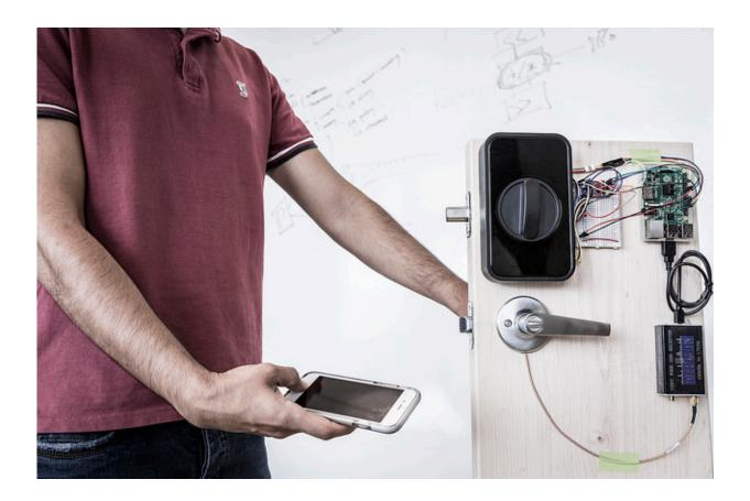
UW engineers use a smartphone to send a secure password through the human body and open a door with an electronic smart lock. These "on body" transmissions employ low-frequency signals generated by the phone's fingerprint sensor. Credit: Mark Stone/University of Washington
