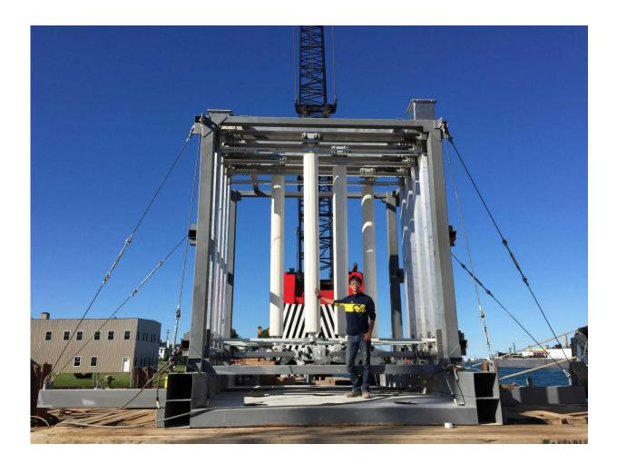
Mechanical engineer Eun Soo Kim with the Vivace device, shortly before its deployment in June of 2016. The indentations on the surface of the cylinders will help water currents push them back and forth, increasing the device's efficiency. Credit: Vortex Hydro Energy
