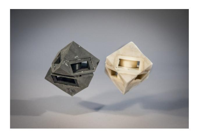
MIT researchers outfitted their cube robot with shock-absorbing "skins" (left) that transfer less than half of the energy that would normally be transferred to the ground. Credit: Jason Dorfman/MIT CSAIL
