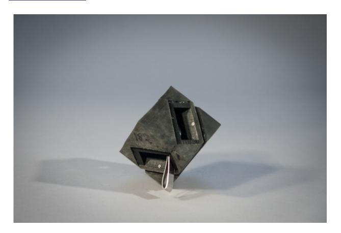
The shock-absorbing skins allow the robot to land more precisely, suggesting that they could be used to help extend the lifespan of delivery drones like the ones being developed by Amazon and Google. Credit: Jason Dorfman/MIT CSAIL
