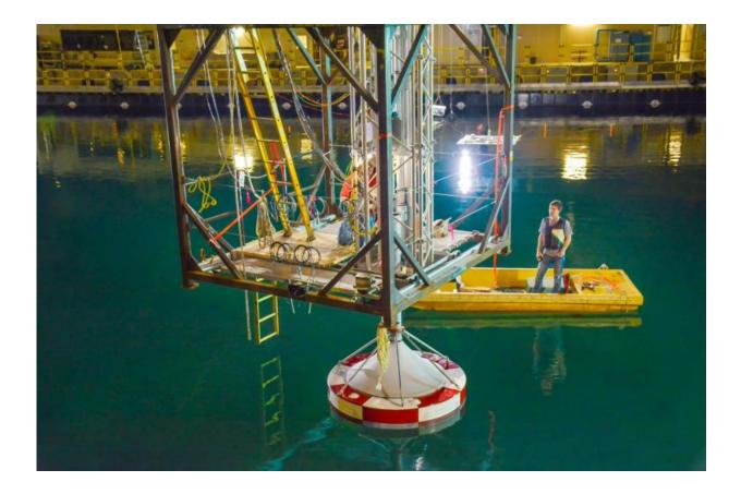
The largest model-scale wave energy testing of its kind is being performed by Sandia National Laboratories at the Navy's Maneuvering and Sea Keeping facility at the Carderock Division in Bethesda, Maryland. Credit: Sandia National Laboratories
