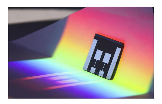
A tandem perovskite solar cell boosts efficiency by absorbing high- and lowenergy photons from the sun. Credit: Rongrong Cheacharoen/Stanford University
