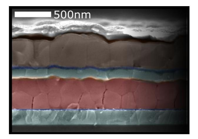
Cross-section of a new perovskite tandem solar cell created by Stanford and Oxford scientists. The front perovskite cell (red) absorbs high-energy light waves, and the rear cell (brown) absorbs lower-energy light. Together, the cells can achieve a 20.3 percent power conversion efficiency. Credit: Giles Eperon
